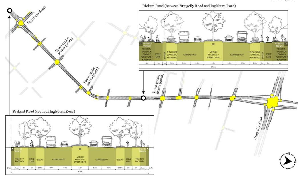
Figure 11: Rickard Road general cross-sections and future model representation between Bringelly Road and Ingleburn Road
