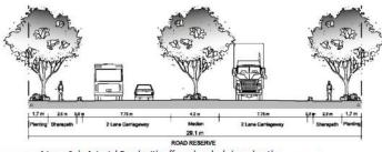
4 Lane Sub-Arterial Road with off road cycle / shared path (source: DCP)
