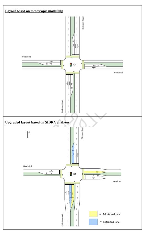
Figure 28: Upgraded layout at Dickson Road / Heath Road intersection
