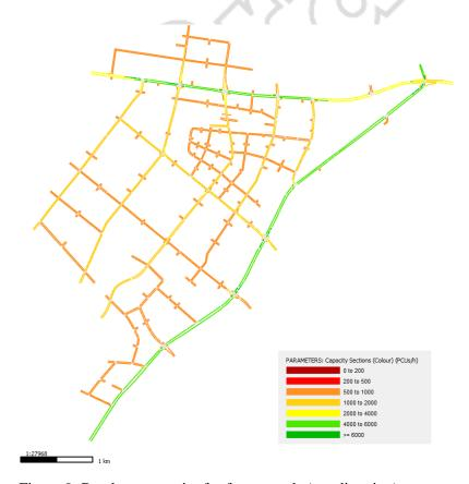
Figure 9: Roadway capacity for future roads (per direction)
