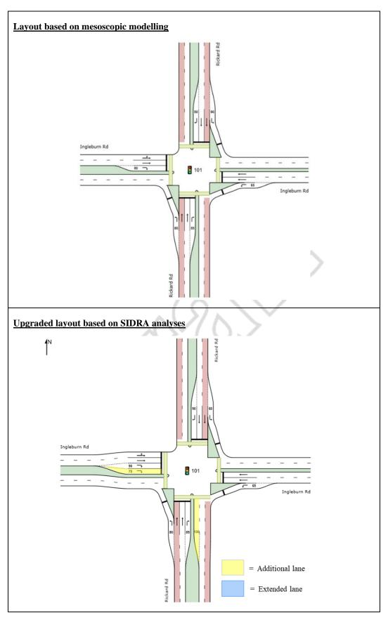
Figure 27: Upgraded layout at Rickard Road / Ingleburn Road intersection
